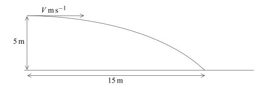
(a) Show that the time it takes for the ball to travel to the point where it hits the ground is 1.01 seconds, correct to three significant figures. (3 marks)
